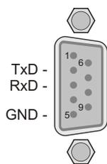
Pin 2: TxD (Transmit Data / output)
