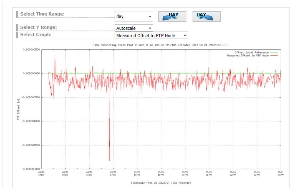
Figure: Graphical diagram of offset values for each node, selectable for different time ranges (day, week, month or manual selection). With given buttons at the "Select Time Range" you can select either past or future intervals for the graphical representation.
