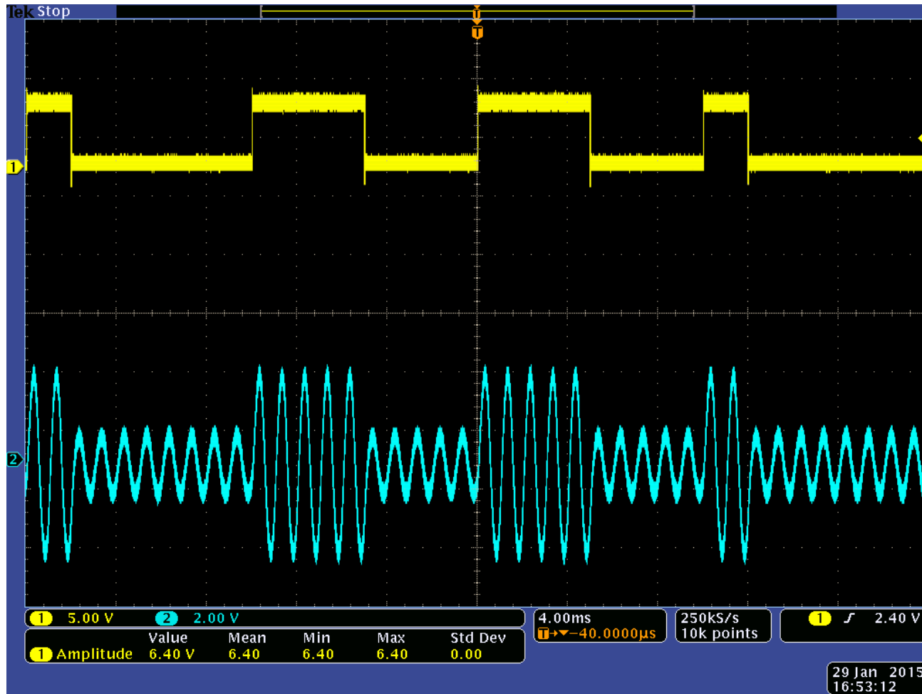
Modulated IRIG signal, 1 kHz carrier frequency
